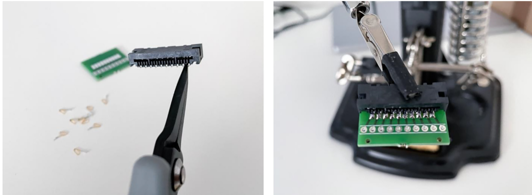
Fig. 2. Removing pins from the mini edge card connector (left) and joining the connector components with solder (right).
