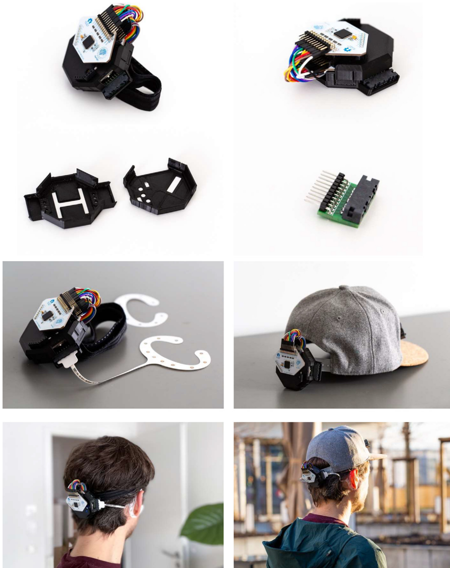
Fig. 1. Overview of the components of the OpenBCI-cEEGrid sensing system. The assembled system and the individual components are shown.
